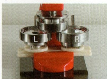
6.Installation complete Place the pattern and badge on the mold to form the finished product
