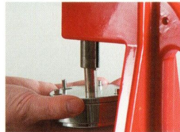
3.The convex points of the upper die are aligned with the grooves of the head and pushed up, and the head will automatically absorb the upper die
