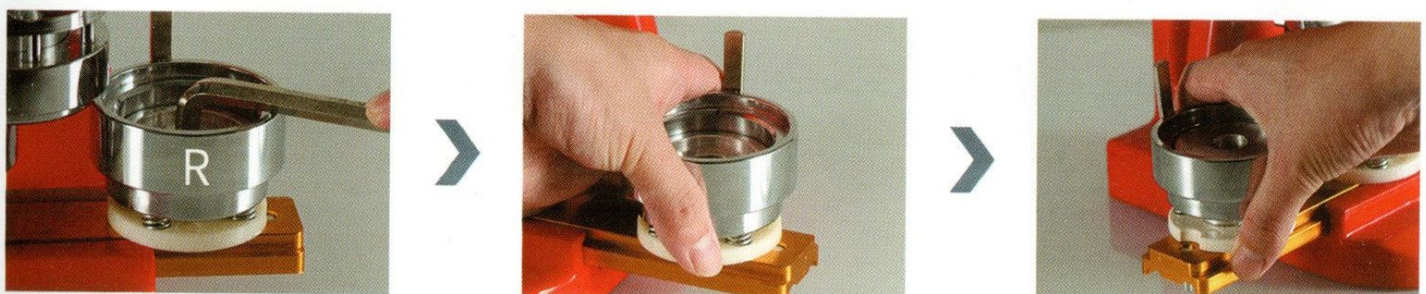
Figure 2: loosen the screw of the mould slightly with a hexagon wrench, rotate the whole die to an angle, and then conduct pressure test until the upper and lower dies are aligned, and then tighten the screws
