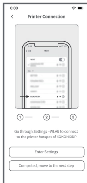
3. Printer hotspot connection: Go through Settings - WLAN to connect to the printer hotspot of (KOKONI3D-xxxx) with the password of 12345678.
