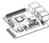
5. Insert one end of the 4 pin cable into the socket of USB expansion board, the other one insert into the socket on the HDMI expansion board.
