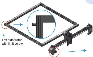
Pay attention to adjusting the eccentric nut to prevent the roller from being damaged by the groove.
