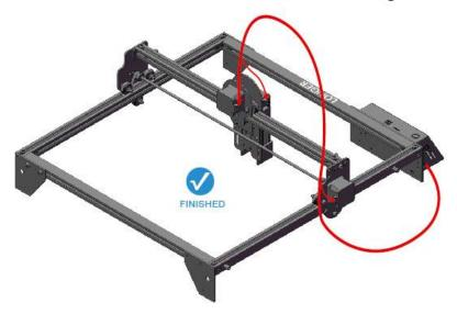
Note: Fix the cable with a cable tie and sheet metal to ensure that the cable has enough length to ensure that the length of the cable is sufficient for the laser head to move to the limit position.
