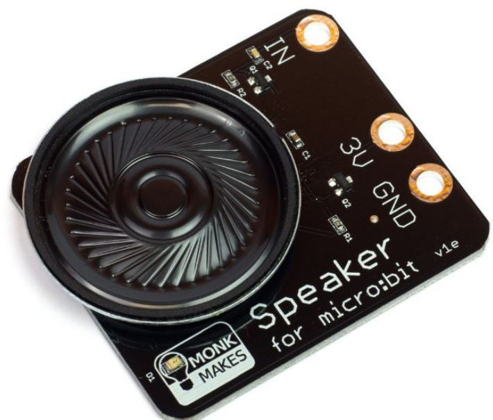
Fig 4: A speaker add-on for the micro:bit which may be used at my club in the future
