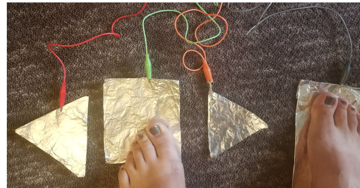
One foot remains stationary on a foil pad clipped to ground; the other foot taps the left, right, and jump "buttons."
