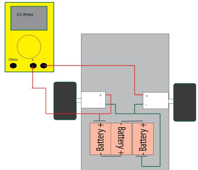
The second motor must also be connected to the power supply and active otherwise only one motor will try to drive the whole Big Trak which will result in an inaccurate measurement. However we only need to measure the current drawn by one of these two identical motors.
