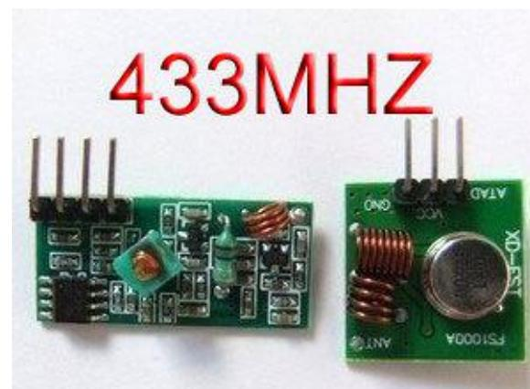
I had to solder a 7" (17cm) antenna wire onto the receiver and transmitter. The antenna length represents a 1/4 wavelength of 433.92MHz. You can use an online calculator such as <http://www.csgnetwork.com/freqwavelengthcalc.html>.
