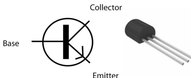
We will be looking at NPN type transistors. This device has three terminals called base, collector and emitter.
