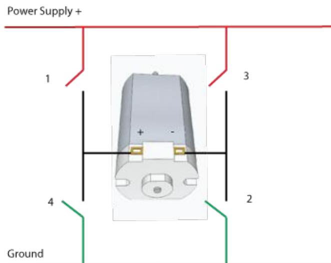
This diagram shows a simplified version of such a circuit. Closing switches 1 and 2 effectively connects the positive rail of the power supply to the + terminal on the motor and ground to the - terminal and the motor runs forwards. Alternatively, closing switches 3 and 4 connects the ground to the + terminal and the positive rail to the - terminal and the motor runs in reverse.
