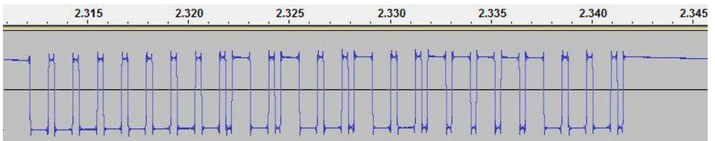
From the waveform I created this binary string. Each bit represents 0.25ms with 1 = high pulse and 0 = low pulse. To aid readability each pulse has been separated with a dash.
