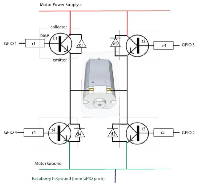
This is then a working H bridge motor controller circuit for a Raspberry Pi (There is a health warning that comes with it however, please take note of it at the end of the article).
