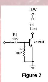
Finally, don't take the power from the GPIO pins, use a separate source - however, you will need to connect the GPIO ground to the buffer ground and, of course, the required GPIO control signal pin to the buffer input.
