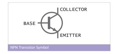
A transistor has three terminals called Collector, Base & Emitter. When a small current is applied to the Base terminal it allows a much larger current to pass between the collector and emitter terminals.
