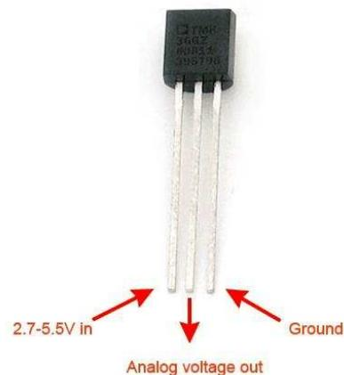
It has a temperature range from  $-40^{\circ}\text{C}$  to  $125^{\circ}\text{C}$  with a typical accuracy of  $\pm 2^{\circ}\text{C}$ . It outputs  $10\text{mV}/^{\circ}\text{C}$  with a  $500\text{mV}$  offset to allow for negative temperatures. To use the chip you read the analogue value and convert this to a voltage between 0 and 5V. The program carries out the necessary calculations to convert the voltage to a temperature in degrees Celsius.
