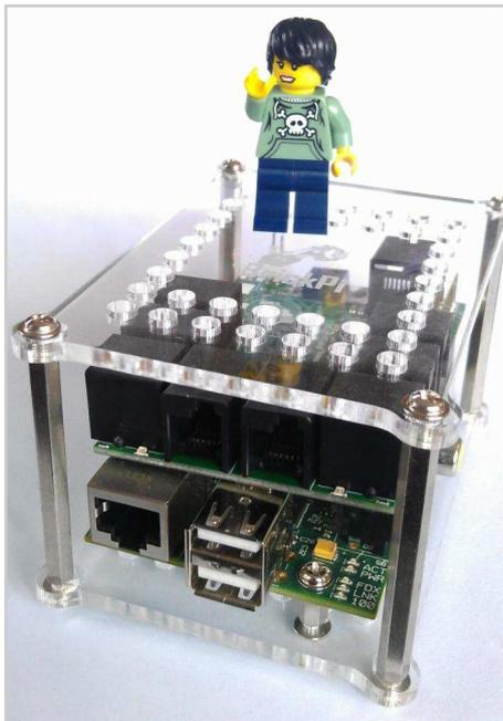
The BrickPi can be used to control up to four LEGO® NXT motors and read the motor encoder values. The motor encoder values
