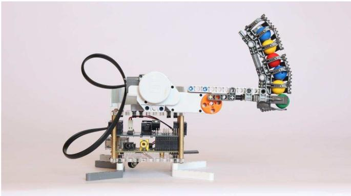
This example shows how to build a turret ball shooter. The turret can rotate and is controlled by the mouse. Moving the mouse left and right changes the angle of the shooter, and the firing mechanism is controlled with a press of the mouse button. A great demonstration in class and fun in the office too.
