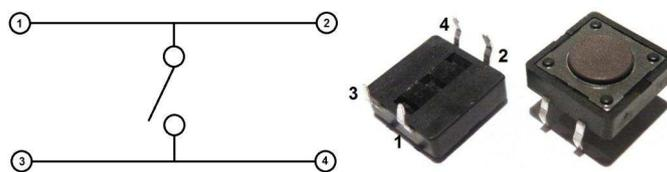
4. Add 10kΩ Resistor. Connect this from Switch Pin 1, to the positive (+) rail of the breadboard. Orientation of standard film resistors is unimportant.
