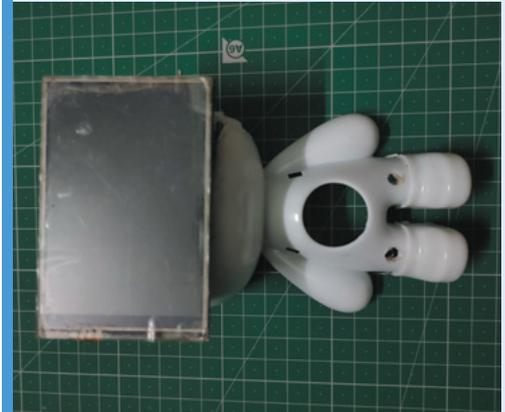
**01** Repurpose or 3D-print a case that will house Raspberry Pi and hold a small touchscreen display in place. Affix the screen to the case.
