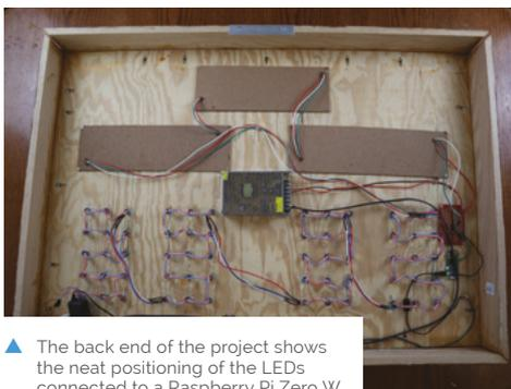
▲ The back end of the project shows the neat positioning of the LEDs connected to a Raspberry Pi Zero W
