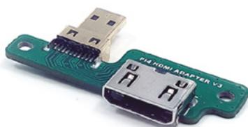
▲ Different, simple adapters need to be used depending on which Raspberry Pi you install
