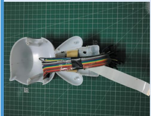
**02** Create a hole for a Camera Module and position it in place. Use jumper wires to connect the screen to your Raspberry Pi.
