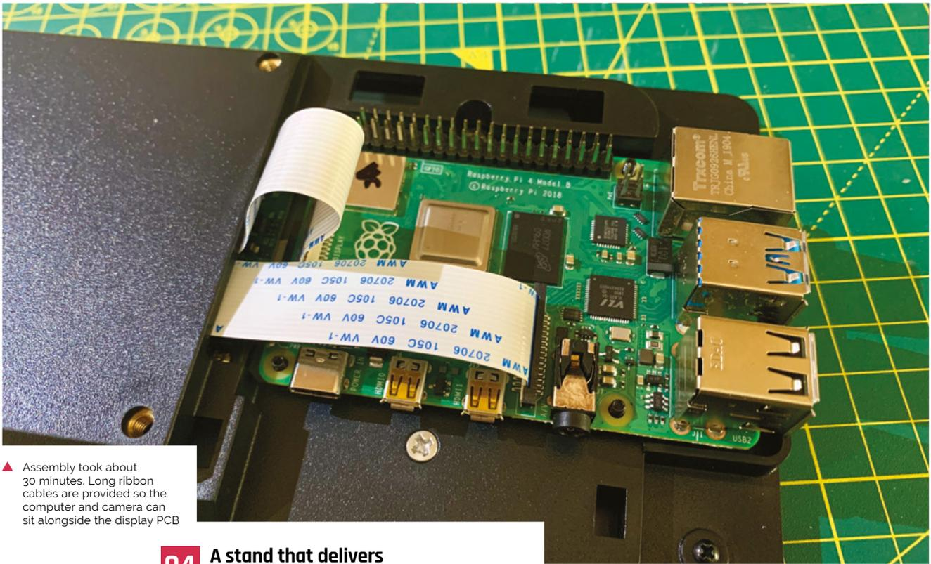
▲ Assembly took about 30 minutes. Long ribbon cables are provided so the computer and camera can sit alongside the display PCB
