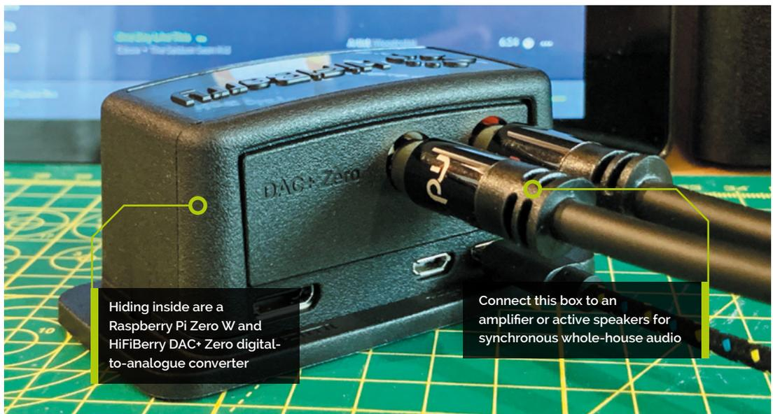
Hiding inside are a Raspberry Pi Zero W and HiFiBerry DAC+ Zero digital-to-analogue converter
