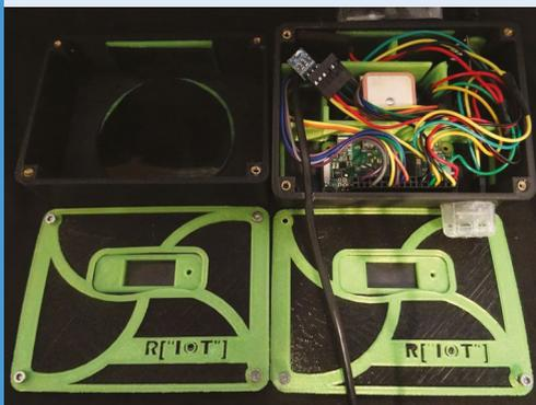
**02** Temperature, pressure, humidity, and light readings are provided by BME280 and BH1750 sensors. Data from all the sensors and transceivers is stored locally in an SQLite database on Raspberry Pi Zero.
