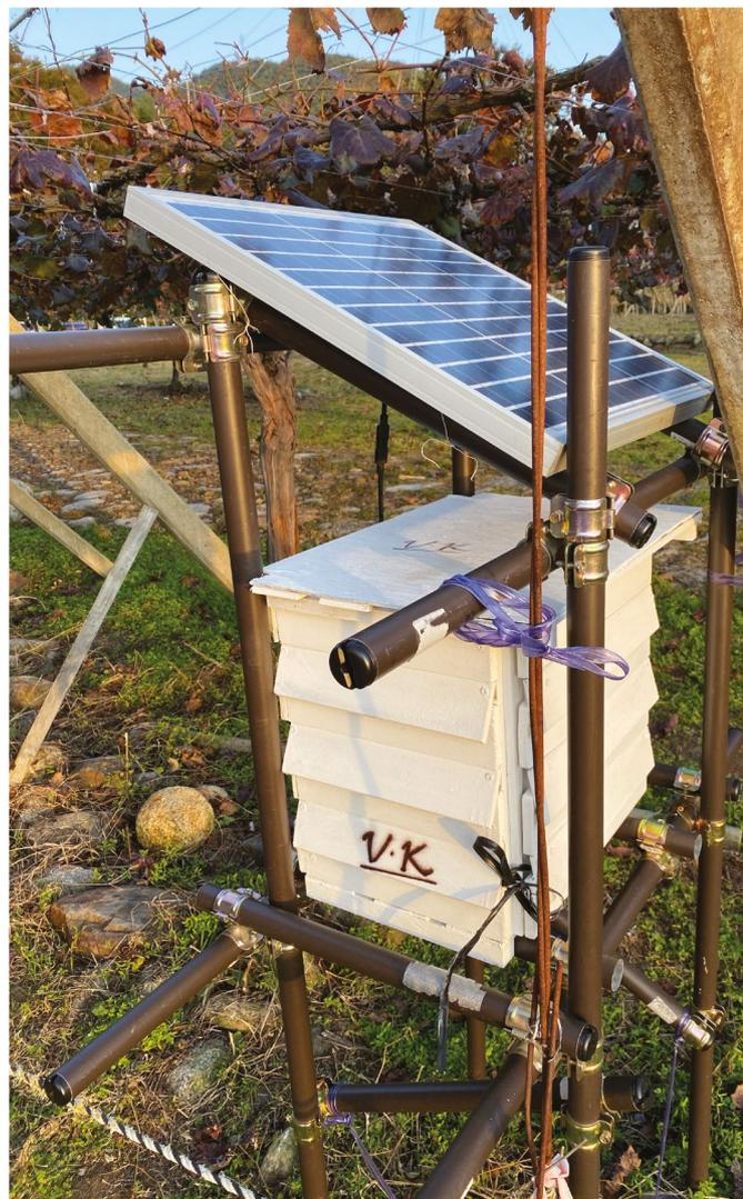
▲ The first prototype system set out in the field. Sensors hang out of the box to obtain an accurate reading
