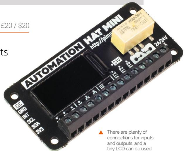
▲ There are plenty of connections for inputs and outputs, and a tiny LCD can be used to show their status
