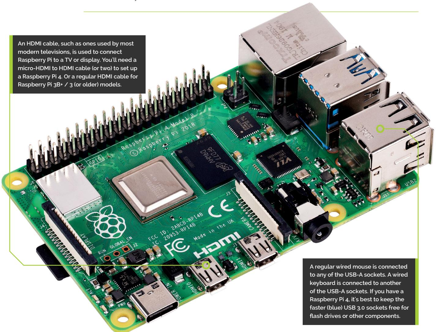
A regular wired mouse is connected to any of the USB-A sockets. A wired keyboard is connected to another of the USB-A sockets. If you have a Raspberry Pi 4, it's best to keep the faster (blue) USB 3.0 sockets free for flash drives or other components.
