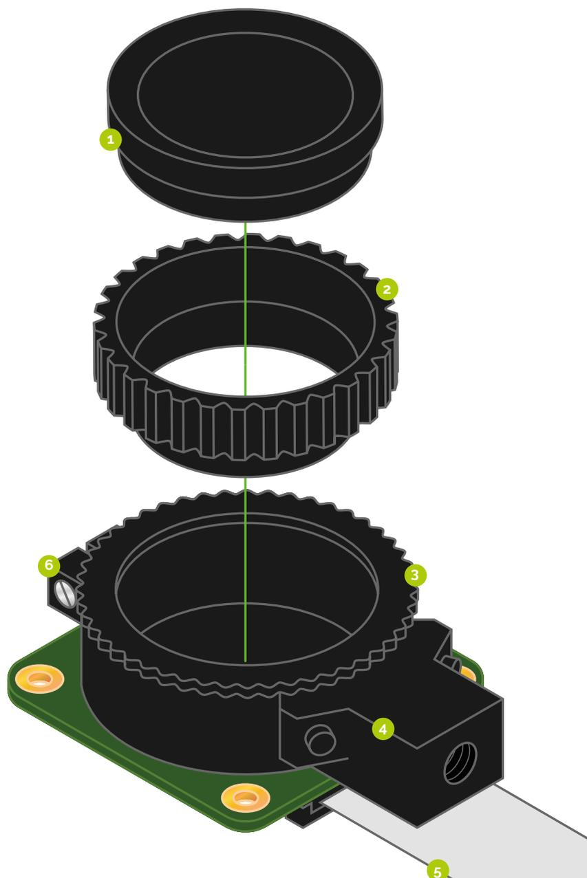
1. The dust cap should be used when a lens is not attached, as the camera sensor is sensitive to dust
