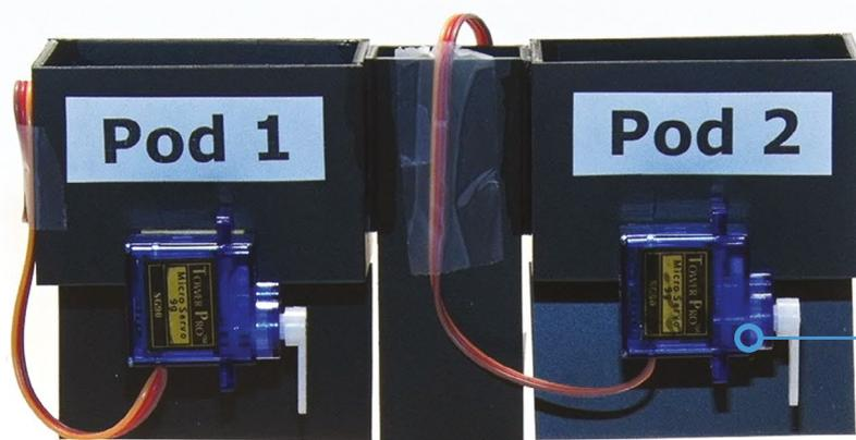
After the doors of the pods open and serve the nuts, the servos stop operating; this reduces wear and power drain
