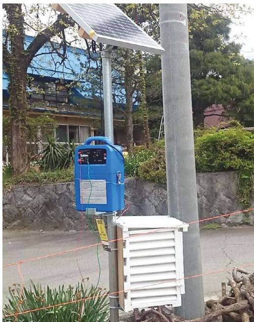
automatically measured at regular intervals,” he explains. “I want to check those data in real-time through the network, as the fields are scattered and far away from my office.” This also means the setup requires solar and battery electric power.
