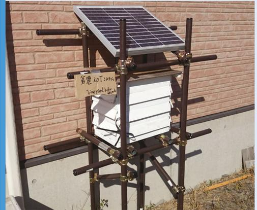
**01** The grapes are monitored from the office using the Hinno IoT system to see what the atmospheric conditions are in the fields.
