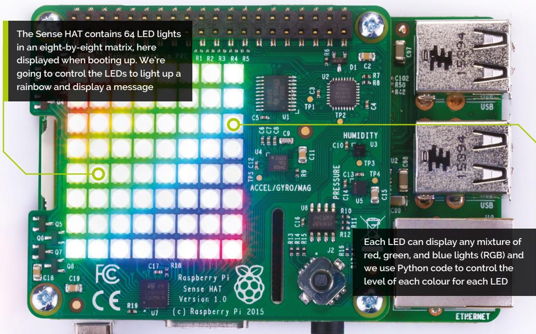
The Sense HAT contains 64 LED lights in an eight-by-eight matrix, here displayed when booting up. We're going to control the LEDs to light up a rainbow and display a message
