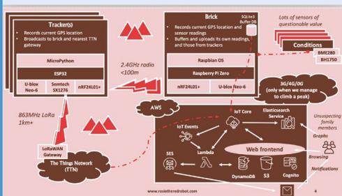
**03** This useful schematic shows the data flow and how to assemble the RIoT Brick. Full instructions are at [magpi.cc/riot10peaks](http://magpi.cc/riot10peaks).
