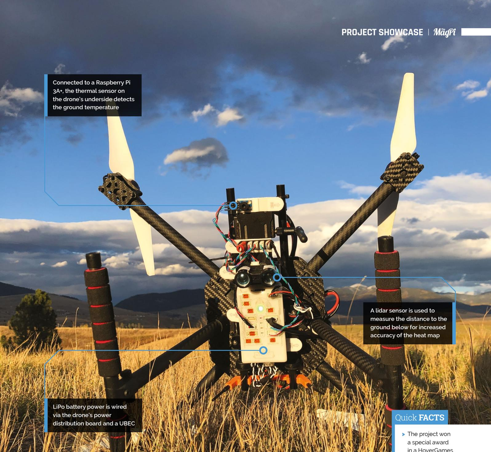
Connected to a Raspberry Pi 3A+, the thermal sensor on the drone's underside detects the ground temperature
