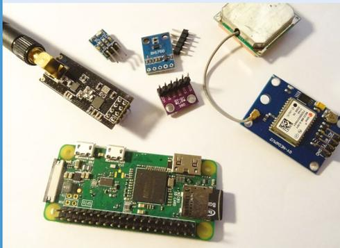
**01** Connect your Raspberry Pi Zero to an nRF24L01+ transceiver. This will receive the data from the other sensors. You also need a u-blox NEO-6 GPS receiver to obtain GPS readings.
