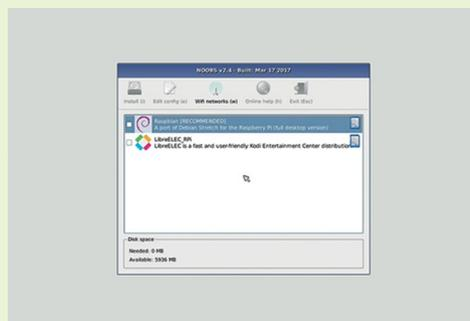
After downloading the NOOBS file to your computer, double-click to unzip it. Then copy all the files from the NOOBS folder to your attached micro SD card. Once done, eject the card and insert it into your Raspberry Pi.
