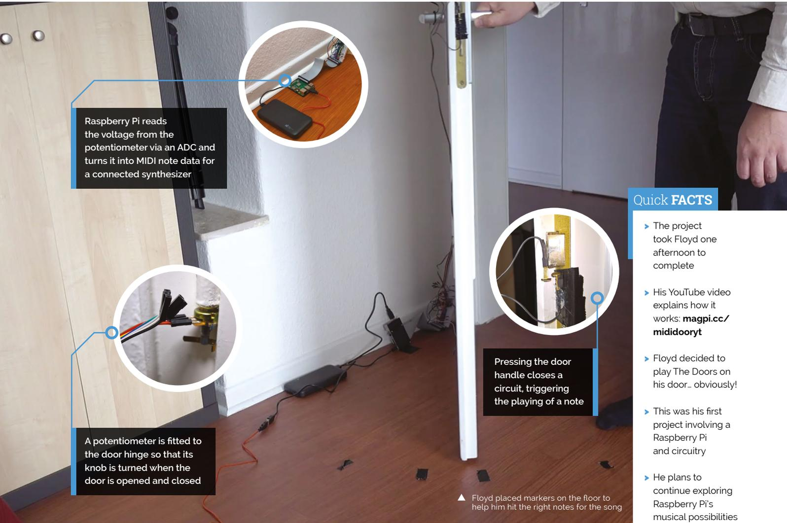
Raspberry Pi reads the voltage from the potentiometer via an ADC and turns it into MIDI note data for a connected synthesizer
