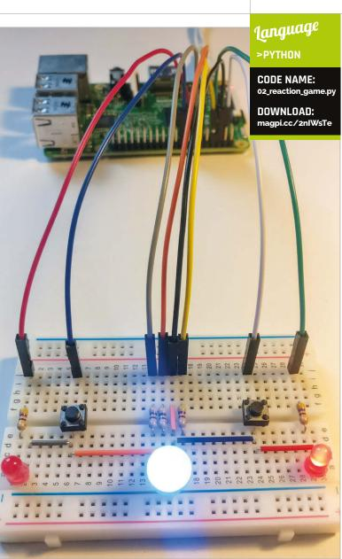
Above For a tidy breadboard, trim the legs of the components and jumper wires so that they sit neatly on the surface
