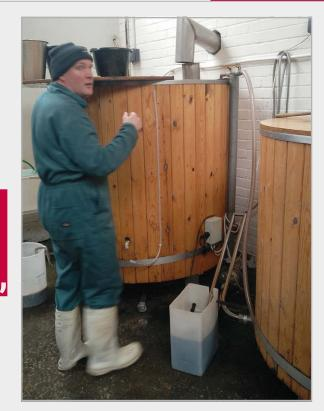
Above Ben transfers the freshly brewed beer to a 'copper' tank, where it will pass through a heat exchange
