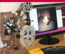
>STEP-02 Client computing Each still frame of the reel is captu one frame at a time. The Raspberr sends the images to a client comp
