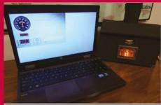
>STEP-01 Temperature set The temperature is set in 25°F (~14°C) increments, starting at about 300-350°F (150-175°C) and is manually increased over 5-6 minutes to 450°F (230°C).
