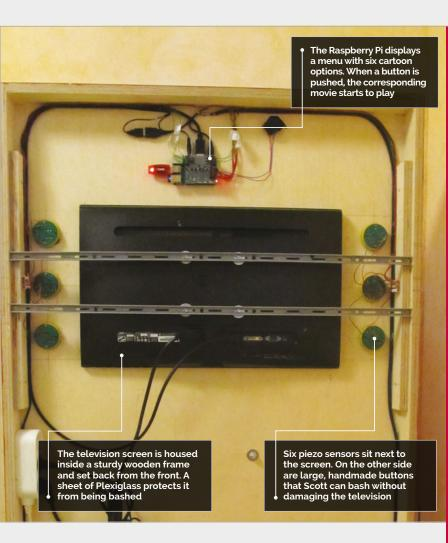
Plexiglass in front of the display is the solution. "It wasn't complicated to build," says Alain. "With a jigsaw, a drill machine, and a little table saw, all is possible.
