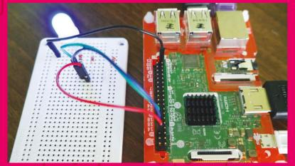
The CPU monitor in action. Chunky 10mm LEDs make a big, bright indicator
