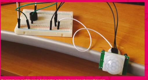
The program uses an infinite loop to detect motion, making the buzzer beep whenever that occurs
