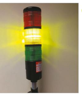
magine being able to show the status of your Jenkins projects to anyone in the same room without the hassle of logging in to the dashboard. With some LEDs, a few other cheap components, and some soldering skills, you can complete this project. You can take it to the next level, however, by using an industrial tower light instead of regular LEDs. Employing an existing API, you can retrieve almost any data from Jenkins and get a nice visual indicator of the status of your project.
