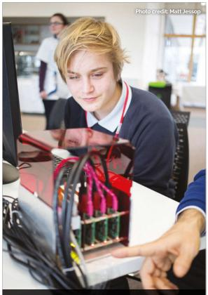
The Grappolo is a small Raspberry Pi supercomputer used to teach cluster computing using a grid engine
