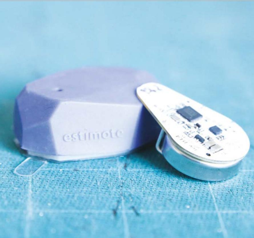
The Estimote beacon transmits a steady ping that can be picked up by the Raspberry Pi
