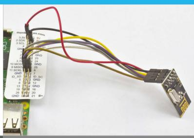
You should wire up the RF module with your Raspberry Pi powered down, and check very carefully that the connections are all correct before you power it back up again. Using a GPIO template like the Raspberry Leaf (by MonkMakes) will help you find the correct connections on the GPIO connector.
