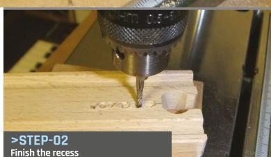
Fit a router bit to the drill and join up the blind holes. Make a smooth recess so that the reed switch can sit flush with the surface of the rail.
