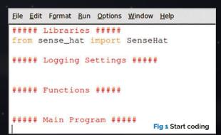
To get data from the Sense HAT, you'll need to write a function called **get\_sense\_data**, which will check each sensor in turn and store the sensor data in a list. The function should be added to the **Functions** section.
