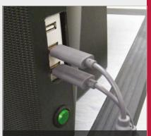
A cheap USB hub was adapted to provide external access to the Pi Zero inside the television
