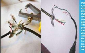
**USB OTG** is a simple extension to the existing micro-USB spec. The connectors are really cheap: under £1 online. That said, it's pretty simple to make your own if you're confident with wiring and soldering. Terence spliced an old one directly into the controller lead
