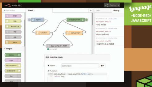
Drag and drop a TCP request node from the function section of the node panel. The server is 127.0.0.1, and the port is 4711. As we're not expecting a return value, we'll Return 'after a fixed timeout' of oms. This connects Node-RED to the *Minecraft* TCP socket – if you're keen to understand what a socket is, have a look at the original workshop material: **magpi.cc/1jLWFST**.
