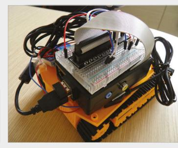
"The next challenge I faced was connecting the UBEC to the Raspberry Pi. I had to find a way to connect the power output wires of the UBEC to the USB connector. Fortunately, I came up with the idea of cutting a USB cable and joining its two internal power cables to the output power cables of the UBEC; this was my real eureka moment."
