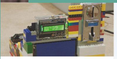
The Raspberry Pi Piggy Bank uses a coin-sorting mechanism to place coins in the correct slots. It counts, sorts and stores coins using a Lego mechanism that rotates for each coin. A fingerprint sensor is used to provide access to the bank.
