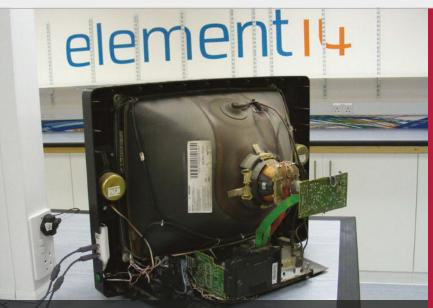
The wires from the Pi Zero are attached directly to the SCART board inside the TV
