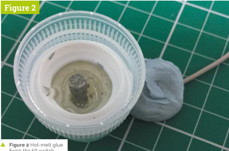
▲ Figure 2 Hot-melt glue fixing the tilt switch
