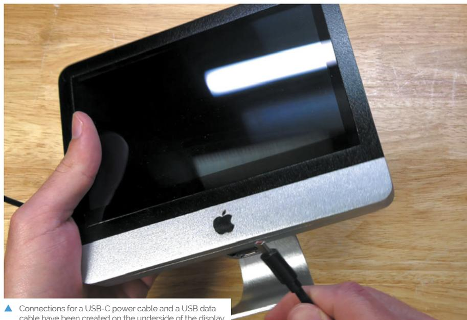
▲ Connections for a USB-C power cable and a USB data cable have been created on the underside of the display
