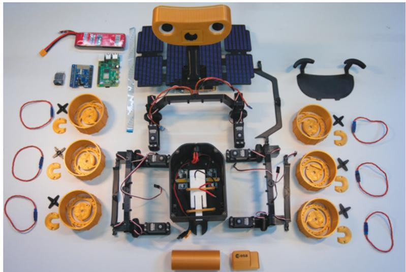
▲ The rover is made from 3D-printed parts and readily available servo motors and screws, plus a Raspberry Pi 4 and Camera Module v2
