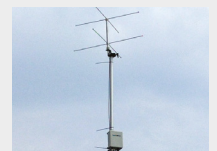
Figure 8 A permanent outdoor static station with a turnstile antenna and waterproof enclosure. Power and network connection are both supplied via a Power over Ethernet (PoE) cable
