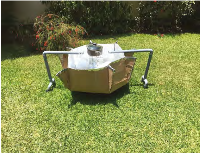
Left ♦ This solar oven can heat food up to 60°C, the minimum temperature needed to kill bacteria
