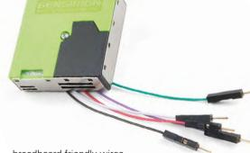
breadboard-friendly wires that are colour coded for simple hook-ups. Sensirion also provides drivers for both the UART protocol and I<sup>2</sup>C. Just keep in mind that if you plan to use this with your Arduino, it works best with UART and not I<sup>2</sup>C. As always, check out the datasheet for more information. Left A high-quality sensor that's fairly easy to use
