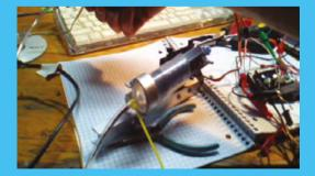
photos and videos. His universal gripper can pick up very irregular or smooth objects easily, despite the fact that it uses off-the-shelf syringes instead of expensive vacuum pumps and reservoirs.
