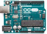
The Arduino Uno controls motors, lighting, cameras, and simple robots, while more powerful models have WiFi and Ethernet. Arduino works through a
