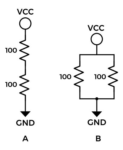
We'll use 5 V for Vcc. What is the total resistance between VCC and GND in each circuit? How much current is flowing through each circuit? What is the voltage across each resistor?
