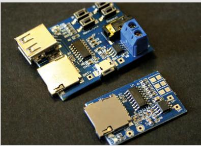
provides flexibility in the field, as does the ability to connect a battery. It just would have been nice to have a JST connector for lithium batteries to connect to, but at this price that would be asking too much. The speaker terminals are handy to have but, in all honesty, 90% of us will just connect an amplified 3.5 mm speaker, so we could desolder those terminals to lower the height of the board, and of course add the terminals to our bits box.
