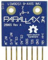
almost any microcontroller, and it can be powered by 2.8, 3.3, or 5 volts. Communication works with either a 3-pin SPI interface or an I<sup>2</sup>C bus, and features an interrupt which can be used for detecting and reacting to free falls or other inputs. It's all ready to use with the BlocklyProp environment, but you can use it with almost any other development environment too.
