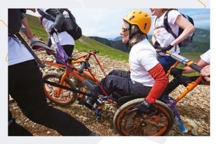
Fred, a retired engineer, looked at the possibility of using a bicycle frame as a removable front wheel for safely steering, braking, and lifting the wheelchair during the challenge. After numerous experiments, a modified BMX bicycle frame was securely fastened to Rosie's wheelchair with U-bolts and pipe clamps, enabling the Women of Altitude team to assemble and disassemble the wheelchair attachment during training sessions quickly. A lifting
