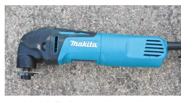
he phrase 'multi-tool' is usually used to refer to a folding pack of knives, screwdrivers, saws, and other gubbins that you can fit in your pocket. What we're looking at here is a completely different beast. Oscillating multi-tools (also known as power multi-
