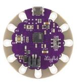
A wearable electronics platform with a built-in microcontroller will be the brains of your circuit. It can read data from sensors, manipulate it, and produce an output. Some popular options for these are the LilyPad USB by SparkFun and the Flora by Adafruit, which are both Arduino-compatible. They come with pins for attaching sensors
