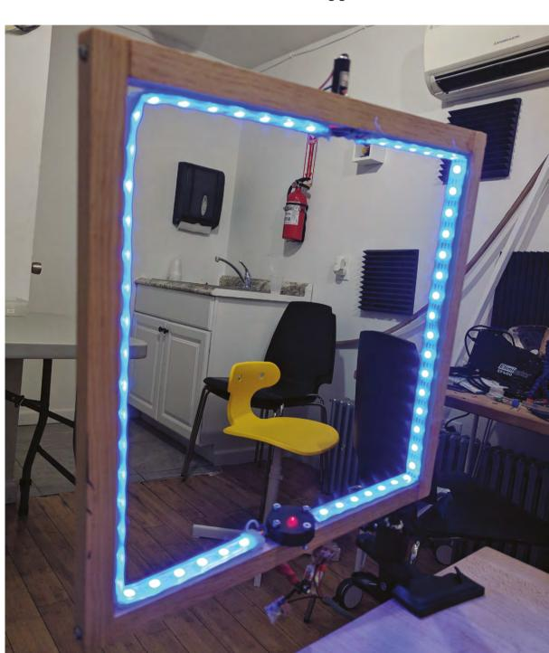
n this tutorial we'll make an Arduino powered laser 'trip-wire' that we can use to build an indoor drone racing game. The end product will be a series of glowing LED gates that can each detect when a drone flies through it (and breaks the laser beam). A gate
