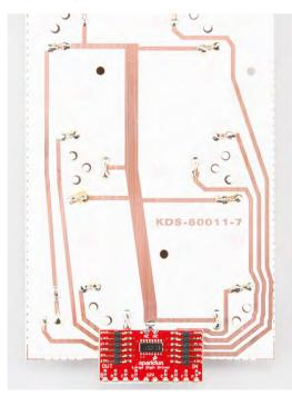
Figure 2 Solder the drivers onto the seven-segment display
