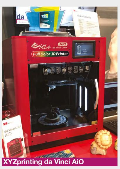
While XYZprinting's closed-source nature is a turn-off, the pricing of its line-up is hard to resist. It unveiled two new products at the show: a 3D printing pen, and a new full colour da Vinci AiO. The da Vinci Color AiO uses an impressive inkjet system to inject colour into the filament as it's being printed. It also contains an integrated 3D scanner, which captures colour in order to create 3D models that take advantage of the colour-printing capability
