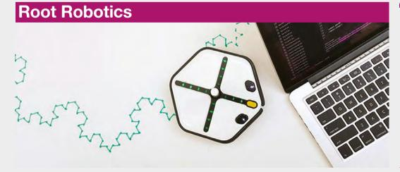
Continuing the theme of teaching kids programming with robots is Root. Root is a little robot that fits in your hand and guides children through coding from graphical to full-text. It's packed with sensors, and even has the ability to drop and lift a pen for drawing. It can also drive on vertical surfaces as long as they're magnetic (like school whiteboards)
