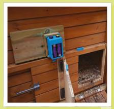
Above The MK2 chicken door, installed on the coop. The battery cover has been removed to show the 18650 batteries inside. This unit is more compact and much easier to set up I 3D-printed a suitable case, and sealed the seams of the unit together using a hot soldering iron. I was feeling quite pleased with the project at this point, and it's a pity that it only worked for three days.
