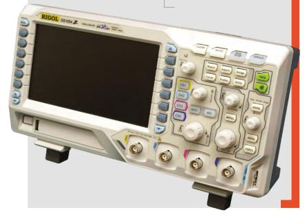
you would see the flat horizontal line move upwards by an amount equivalent to its voltage. So for example if the voltage selector is set to 1 volt per centimetre and a 9V battery is connected, its voltage can be measured through the 9 cm by which the line moves up the screen.
