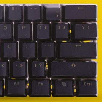
we did looking into how to assemble a keyboard, but with hubris we set about soldering the switches into the PCB. About half way through, we discovered that you have to put the switches into the stainless steel backing plate before soldering them into the PCB. A bit of impromptu desoldering practice later, we started again. The correct order for assembling the keyboard is:
