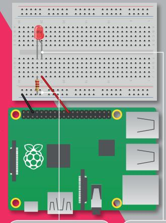
A resistor is used to prevent the LED from burning itself out. The smaller the resistor, the brighter the light will be, but don't burn your LED out. A 330Ω resistor is a good start, though you can use other sizes. However, if you pick one that's too high, you may not be able to see the LED
