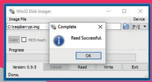
Above: You can clone your SD card to an image file using dd on a Mac or Linux, and Win32 Disk Imager on a PC
