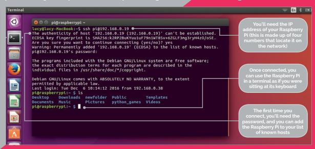
ecure Shell (better known as 'SSH') is an encrypted networking technology that enables you to manage computers from the command line over a network.
