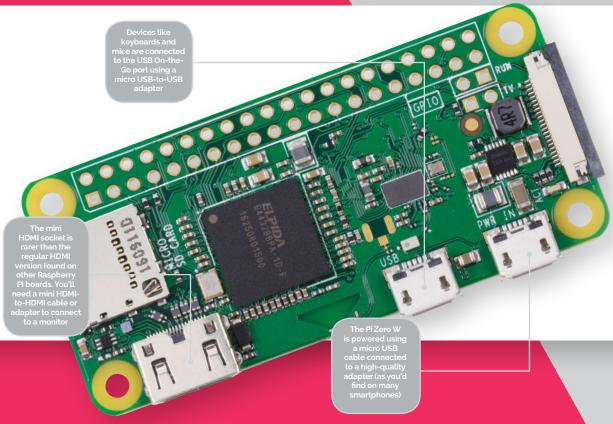
smaller than a regular one. You'll need a micro USB-to-USB adapter to connect your keyboard. You may also want a USB hub to connect
