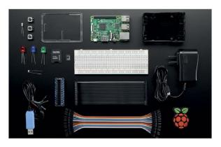
Electronic components are plugged into the holes on the breadboard, and components in adjacent holes are linked. In this way, you can build up a test circuit without having to actually solder components together.
