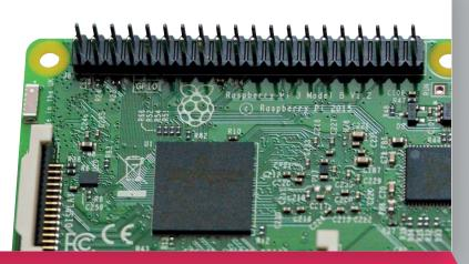
While it's possible to wire parts directly to the GPIO pins, most tinkerers place electronic components in a breadboard and connect this to the Raspberry Pi. Unlike the type used for cutting bread, an electronic breadboard is a plastic slab with lots of holes in it.
