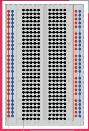
A hole in the blue (sometimes black) rail is connected to a GND pin. It then becomes the ground rail
