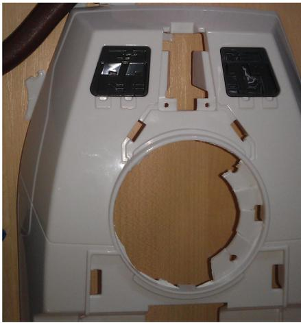
For complete perfection, score around the edge of the hole with a stanley knife or similar and then use a pair of wire snippers to cut out and break off sections of the lip around the turret hole.
