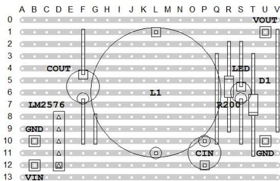
Care should be taken to ensure that there are no short-circuits caused by solder bridging adjacent strips of the stripboard. After you have built and tested the supply, if you are going to connect it directly to the Pi, it should be connected via the 2 points marked TP1 and TP2, with the positive feed going to TP1.
