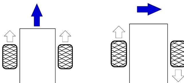
When the wheels are turning in the same direction, the robot will move in that direction. If the wheels rotate in different directions then the robot will turn.
