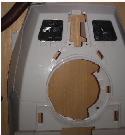
For complete perfection, score around the edge of the hole with a stanley knife or similar and then use a pair of wire snippers to cut out and break off sections of the lip around the turret hole.
