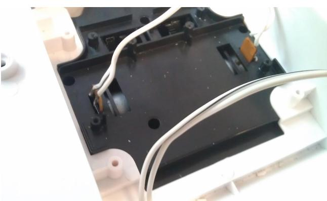
Snip off the wires that are attached to the motors. Solder two double core "bell wire" type cables to each + and - terminal on the two motors.
