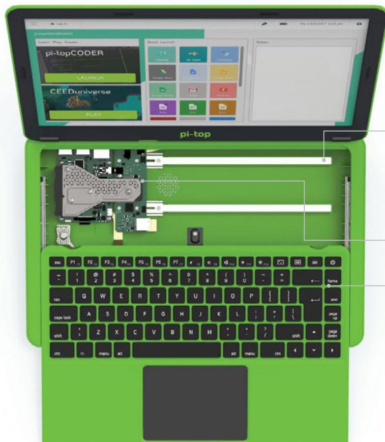
Two magnetic rails are used to quickly connect and remove components to the kit
