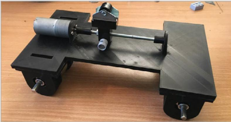
**Above** A long threaded bar converts motor rotation into lateral movement to tilt the whole firing mechanism (not shown) up or down for aiming purposes
