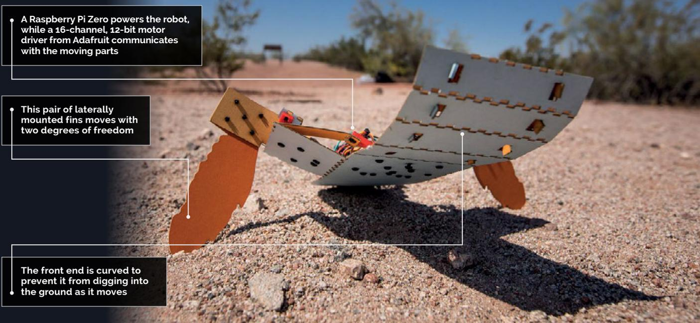
A Raspberry Pi Zero powers the robot, while a 16-channel, 12-bit motor driver from Adafruit communicates with the moving parts
